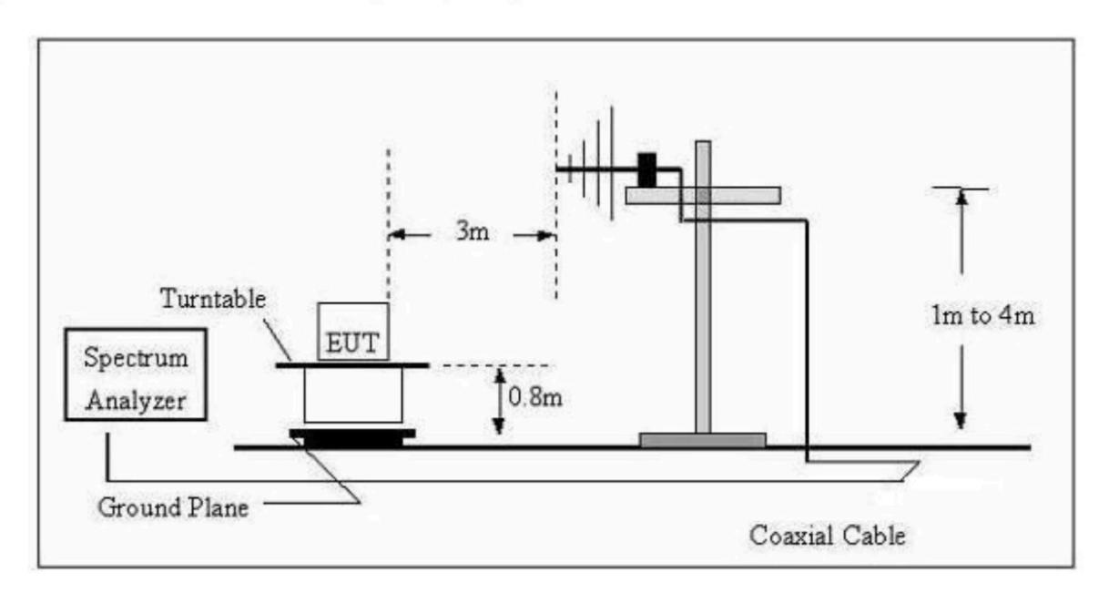
(B) Disturbance Power Test Set-UP Frequency Below 1GHz
