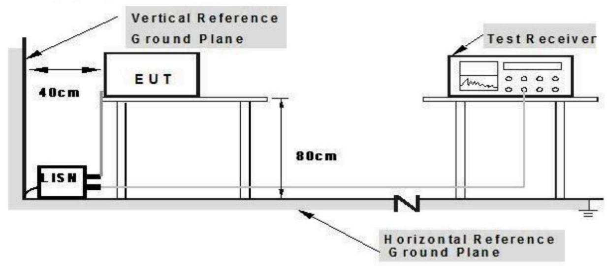
Note: 1. Support units were connected to second LISN. 2.B oth of LISHs (AMN) are 80 cm from EUT and at least 80 from other units and other metal planes
